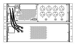
The example at left shows one battery pack properly connected to the UPS. Note that the rear connector plug in the Battery Pack is not removed.
