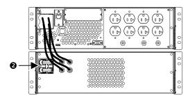
2. Insert the battery pack connector into the rear connector ② on the back of the other battery pack.
