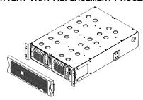
The battery trays are accessible from the front of the battery pack. This procedure requires a Phillips screwdriver.
