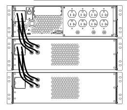
The example at left shows two external battery packs properly connected to the UPS.
