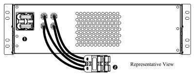
Battery Pack Connector Use the battery pack connector **①** to daisy-chain multiple battery packs to the same UPS. The connector is color-coded and keyed to prevent improper connection.
