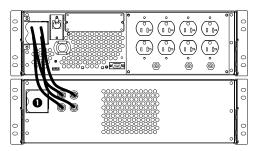
1. When more than one battery pack is used, remove the rear connector plug • from the battery pack connected to the UPS.
